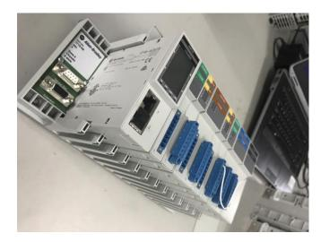
The image to the left shows a 1719-A8 chassis without the required separation plate.
