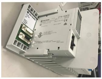
This image shows a 1719-A8 module with the separation plate correctly installed between the 1719-AENTR module and the first I/O module.
