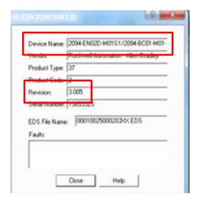
The module identification information can be found on the Device Properties dialog. The product catalog number will be in the Device Name field and the as installed firmware version will be in the Revision field.
