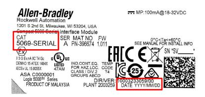
For installed product, the product identification information may be found on the product nameplate. The catalog number is in the CAT field. The date of manufacture is in the DATE field and is of the format YYYY/MM/DD where YYYY is the year, MM is the month number, and DD is the day of the month. For example, 2019/11/10 is November 10, 2019.
