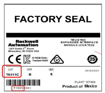
For product still in its shipping carton, the product identification information is found on the carton label. The catalog number is in the lower left in the CAT field and the manufacturing date code will be the first five characters of the serial number, located under the serial number bar code in the lower left corner.
