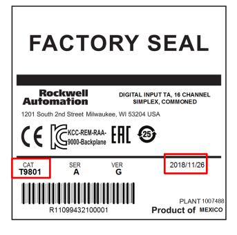
For AADvance product still in its original carton, the product identification information will be on the product carton label. The catalog number will be in the "CAT" field and the date of manufacture will be on the right side under the dividing line and will be of the format YYYY/MM/DD where YYYY is the year, MM is the month code, and DD is the day of the month.
