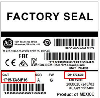
For 1715 Redundant I/O product still in its original carton, the product identification information will be on the product carton label. The catalog number will be in the "CAT" field and the date of manufacture will be in the lower right corner above the "DIR/VER" field will be of the format YYYY/MM/DD where YYYY is the year, MM is the month code, and DD is the day of the month.
