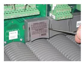
2. Find the **open fuse** and remove it. Rockwell Automation recommends the use of catalog number T9908 fuse removal tool or equivalent long nose pliers. Pull the fuse slowly straight out to prevent damage to the fuse holder.
