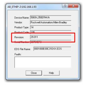
The currently installed version of firmware can be determined using Rockwell Automation network tools, such as FactoryTalk® Linx™ or Studio 5000 Logix Designer®.
