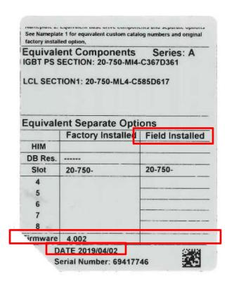
Date of manufacture and firmware information may also be found on the label located under the human interface module (HIM). The date of manufacture is in the DATE field and the as shipped firmware is in the Firmware field. In addition, firmware updates may be shown in the Field Installed column.
