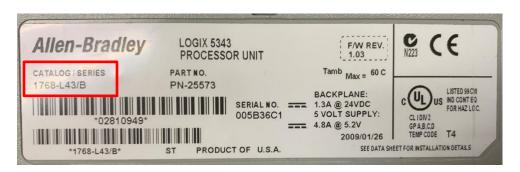
CompactLogix and Compact GuardLogix processors are shipped with default firmware. Operational firmware must be downloaded and installed prior to use. The currently installed processor firmware version can be found on the processor's information or property dialog as viewed in Rockwell Automation network tools, such as RSLinx® RSWho or FactoryTalk® Linx Browser.
