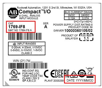
For open and installed product, the product identification information will be found on the module nameplate, located on the side of the module. The catalog number will be in the CAT field and the date of manufacture will be in the lower right corner in the DATE field. The date will be of the format YYYY/MM/DD, where YYYY is the year, MM is the month code, and DD is the day of the month.
