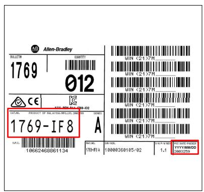
For product distributed in a multi-pack carton, the product identification will found on the distribution label. The catalog number will be in the CAT.NO. field and the date of packaging will be in the bottom right corner in the PKG DATE/PICKER field. The date will be of the format YYYY/MM/DD, where YYYY is the year, MM is the month code, and DD is the day of the month.
