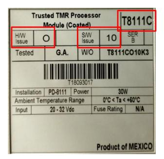
The product catalog number and version information can be found on the product nameplate, located on the side of the module. The catalog number is located in the top right corner and the version number is a combination of the HW Issue letter and the S/W Issue number.
