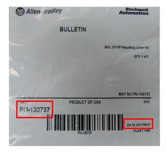
Each affected PanelView product will contain within its shipping carton one or more Bulletin 2711P Mounting Lever kits, with each kit containing 4 mounting levers. Kits contained within PanelView product may be identified by the part number PN-130737, shown in the CAT field on the packaging plastic bag. The date of manufacture will be in the DATE field and is of the format YYYY/MM/DD where YYYY is the year, MM is the month code, and DD is the day of the month.
