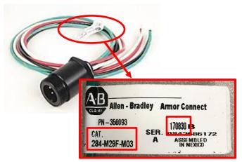
The product identification tag is affixed to one of the product wires and will show the catalog number in the CAT field and the manufacturing date code above the serial number. The date code is in the format of YYMMDD where YY is the last two digits of the year, MM is the month code, and DD is the day of the month.
