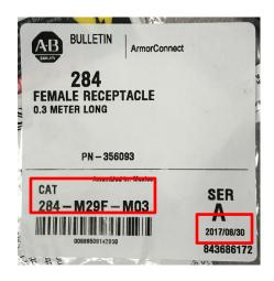
For unopened product still within the packaging bag, the product identification information is on the packaging label. The catalog number is in the CAT field and the manufacturing date is under the SER field and is of the format YYYY/MM/DD where YYYY is the year, MM is the month code, and DD is the day of the year.
